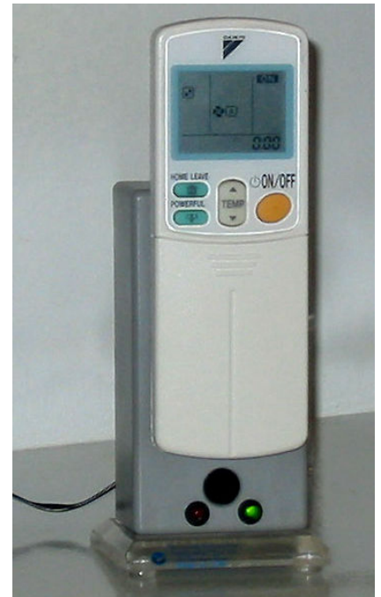
Air Conditioner Remote Control IR Interface:
