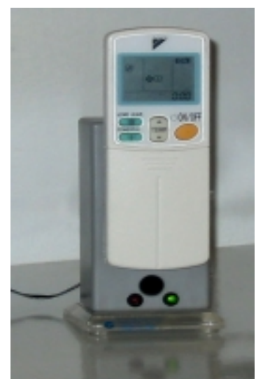
This unit receives a simple IR signal from an ECU and activates the airconditioner remote, which in turn emits its own codes.
